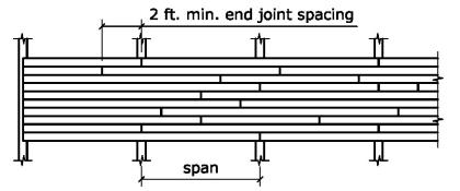
Use a minimum distance of 2 ft. between end joints in adjacent courses. The pieces in at least the first and second course, and repeating at least after each group of seven courses, must bear on at least two supports with end joints in these two courses occurring in alternate spans or on alternate supports.
